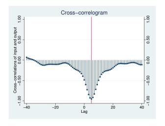
We included a vertical line at lag 5, because there is a well-defined peak at this value. This peak indicates that the output lags the input by five periods. Further, the fact that the correlations are negative indicates that as input (coded gas rate) is increased, output (% CO<sub>2</sub>) decreases.
