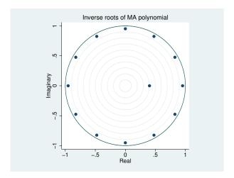
Because the modulus of each eigenvalue is strictly less than 1, the MA process is invertible and can be represented as an infinite-order AR process.
