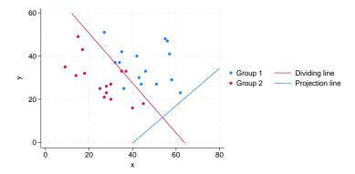
Another way of thinking about the discriminant function is that it projects the data from the original two dimensions down to one dimension—the line perpendicular to the dividing line. Classifications are based on which side of the separating line the observations fall.
