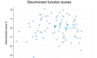
The score plot illustrates the separation due to the first and second canonical linear discriminant functions. As expected from our examination of the earlier descriptive output, the high school group (labeled H) is reasonably well separated from the college (labeled C) and nonplayer (labeled X) groups. There is some separation in the second dimension between the college and nonplayer groups, but with substantial overlap.
