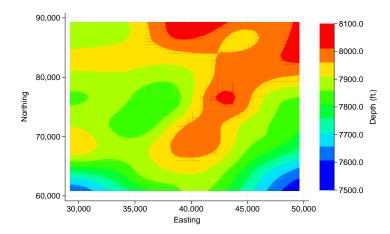
. twoway contour depth northing easting, levels(10) zlabel(#7, format(%9.1f))
