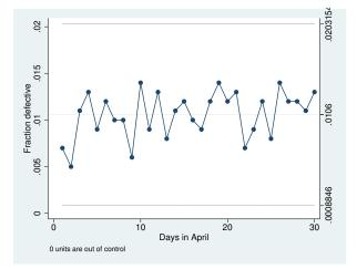
All the points are within the control limits, which are 0.0009 for the lower limit and 0.0203 for the upper limit.
