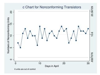
The expected number of defects is 10.6, with lower and upper control limits of 0.8327 and 20.37, respectively. No units are out of control.
