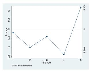
If we also know that the standard deviation of the process is 0.3, we could type . xchart m1-m5, connect(1) mean(11) std(.3)
