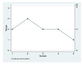
The expected range in each sample is 2 with lower and upper control limits of 0 and 4.23, respectively. If we know that the process standard deviation is 0.3, we could specify
