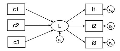
In this model, the observed causes c1, c2, and c3 determine latent variable L, and L in turn determines the observed indicators i1. i2. and i3.
