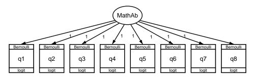
In the 1-PL model, we place constraints that all coefficients, the factor loadings, are equal to 1. The negative of the intercept for each question will then represent the difficulty of the question:
