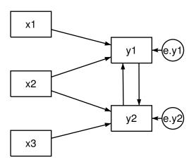
It could be written in command syntax as (y1<-y1 x1 x2) (y2<-y2 x2 x3).
