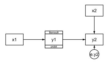
In the command syntax, we could write this model as (y1 < -x1, probit) (y2 < -y1 x2). (In this case, the observed values and not the expectations are used to fit the y1->y2 coefficient. In general, this is true for all generalized responses that are not family Gaussian, link identity.)
