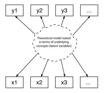
Because the measurement model is so often joined with other models, it is common to refer to the coefficients on the paths from latent variables to observable endogenous variables as the measurement coefficients and to refer to their intercepts as the measurement intercepts. The intercepts are usually not shown in path diagrams. The other coefficients and intercepts are those not related to the measurement issue.
