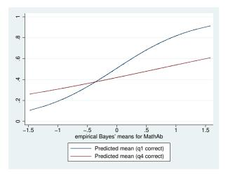
Here the curves are not parallel because the discrimination has not been constrained to be equal across the questions. Question 1 has a steeper slope, so it is more discriminating.
