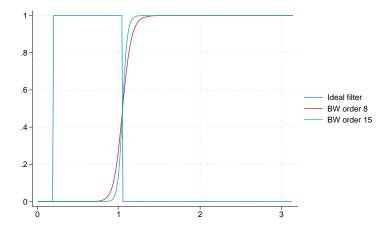
We specified much higher orders for the filter in this example because the cutoff period is 6 instead of 32. (As previously mentioned, holding the order of the filter constant, the slope of the gain function at the cutoff period decreases when the period decreases.) The above graph indicates that the filter with order(15) is reasonably close to the gain function of the ideal filter.
