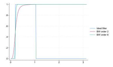
As discussed in [TS] tsfilter, the gain function of the ideal filter is a square wave with a value of 0 at the frequencies corresponding to unwanted frequencies and a value of 1 at the desired frequencies. The vertical lines in the gain function of the ideal filter occur at  $\pi/16$ , corresponding to 32 periods, and at  $\pi/3$ , corresponding to 6 periods. (Given that  $p=2\pi/\omega$ , where p is the period corresponding to frequency  $\omega$ , the frequency is given by  $2\pi/p$ .)
