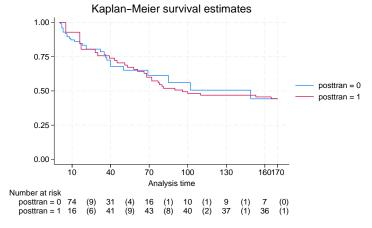
The number of failures for the last interval reported by sts graph is 0 in the first group and 1 in the second group, whereas sts list reported 2 and 18, respectively. We specified tmax(170) with sts graph to restrict the range of the observed times to the maximum of 170, whereas sts list used the observed maximum times for each group (1,400 and 1,799). If we want to match the numbers of failures, we could specify tmax(170) with sts list:
